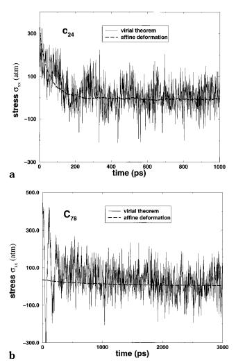
**Figure 6.** Evolution of the component  $\sigma_{xx}$  of the stress tensor with time t for (a) the  $C_{24}$  and (b) the  $C_{78}$  PE melt systems. The results at every time t have been obtained by applying either the virial theorem and averaging over all dynamical trajectories (thin solid line) or by using the thermodynamic expression, eq 25, as explained in the text (thick broken line). Simulation conditions: T = 450 K,  $P_{\text{ext}} = 1 \text{ atm.}$
