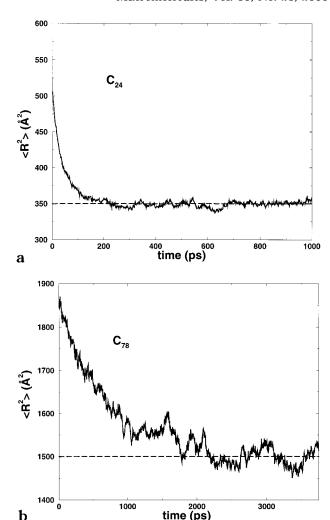
Figure 2. Time evolution of the mean-square chain end-toend distance  $\langle {\it R}^2 \rangle$  for (a) the  $C_{24}$  and (b) the  $C_{78}$  PE melt systems, averaged over all  $NTL_x\sigma_{yy}\sigma_{zz}$  trajectories (T=450 K,  $P_{\text{ext}} = 1$  atm). The dashed lines in the figures show the equilibrium values of the mean square chain end-to-end distance  $\langle R^2 \rangle_0$  for the two systems, obtained by EBMC or *NVT* MD equilibrium simulations.
