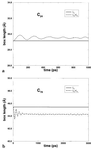
**Figure 3.** Time evolution of the lengths  $L_x$  and  $L_y = L_z$  of the simulation box, as obtained from averaging over all simulated trajectories for (a) the  $C_{24}$  and (b) the  $C_{78}$  PE melt systems (T  $= 450 \text{ K}, P_{\text{ext}} = 1 \text{ atm}$ ).
