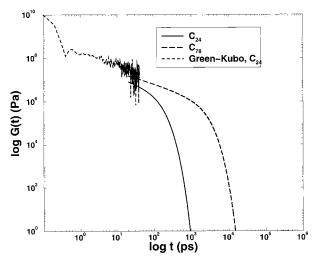
**Figure 8.** Relaxation modulus G(t) for the  $C_{24}$  and the  $C_{78}$  PE chain systems. The curves have been reconstructed by using eq. 26 with the values of  $\tau_R$  obtained by mapping the simulation results onto the Rouse model. G(t) for  $C_{24}$ , as calculated directly from the Green–Kubo expression, is shown as a broken line on the left-hand side, short time region of the figure. (T=450 K,  $P_{\rm ext}=1$  atm).
